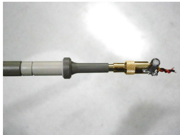
Figure 42 – Oscilloscope Probe with Probe Master ( www.probemaster.com ) 4901-2 BNC Adapter. (Modified with wires for ripple measurement, and two parallel decoupling capacitors added)
