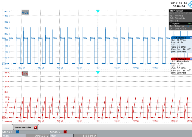
Figure 23 – 90 VAC, Full Load. Upper: V_{DS} , 50 V / div., 50 \mu s / div. Lower: I_{DS} , 400 mA / div., 50 \mu s / div. V_{DS(MAX)} = 306.72 V. I_{DS(MAX)} = 1.6316 A.
