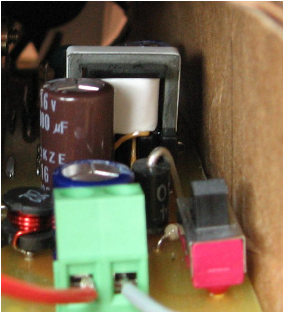
Figure 54 – Standby Transformer T2, Visible Light View.
