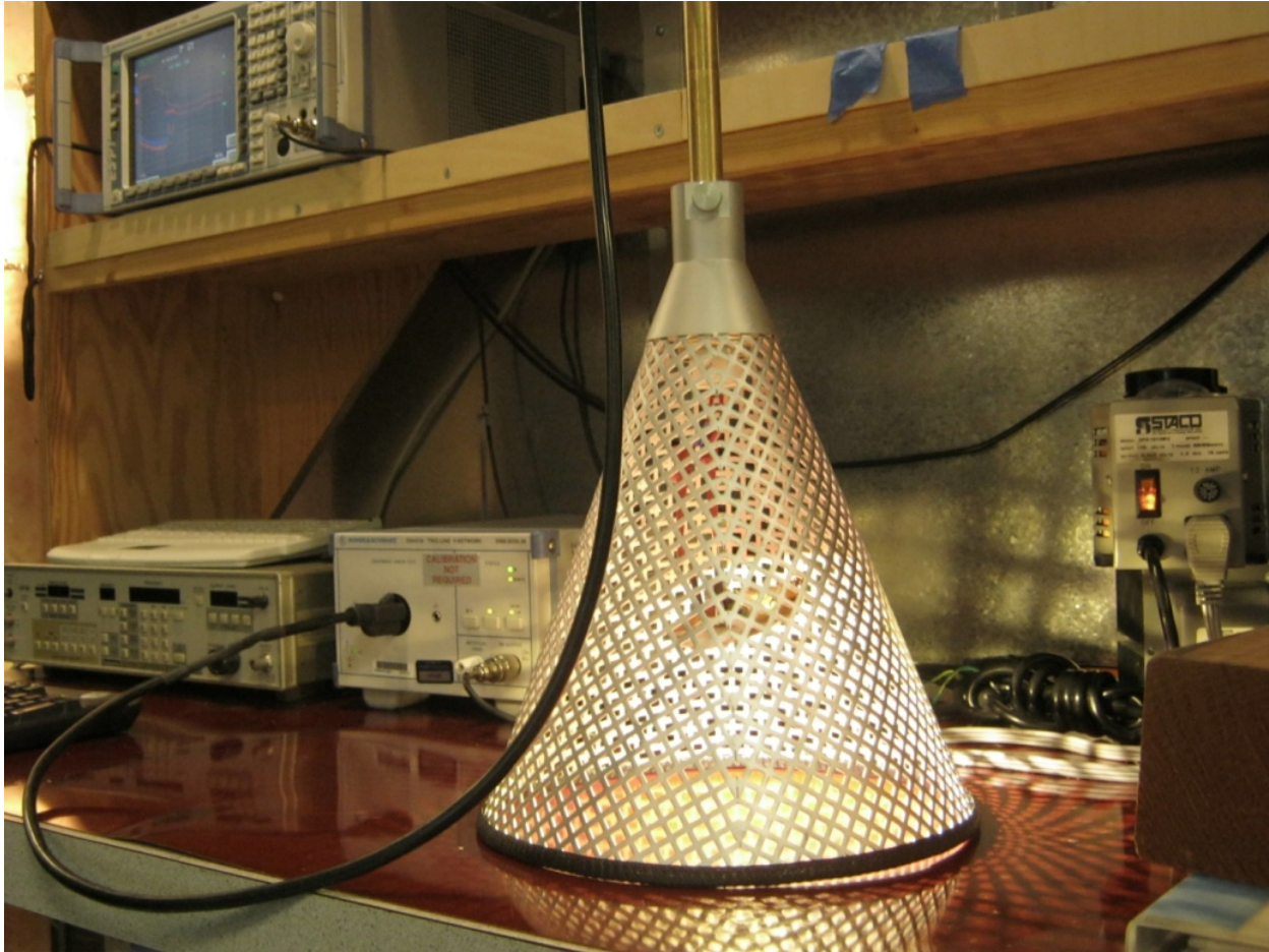
Figure 46 – EMI Test Set-up with the Unit and LED Load Placed Inside a Conical Metal Housing as Described in CISPR 15 / IEC: 2005 Standard.
