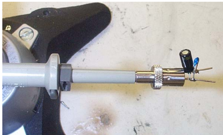
Figure 46 – Oscilloscope Probe with Probe Master 5125BA BNC Adapter. (Modified with wires for probe ground for ripple measurement, and two parallel decoupling capacitors added)
