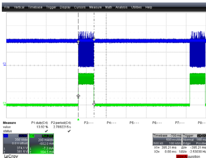
Figure 52 – 265 VAC Input and Maximum Load. Upper: V_{DRAIN} , 200 V / div. Lower: I_{DRAIN} , 0.2 A, 20 \mu s / div. Auto-restart On Time, 395 ms. Auto-restart Off Time, 2.4 s
