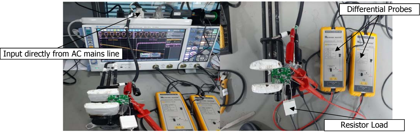
Figure 73 – ZCD Voltage Measurement Set-up.
