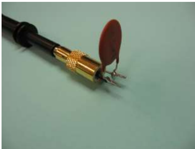
Figure 67 – Oscilloscope Probe with Probe Master ( www.probemaster.com ) 4987A BNC Adapter (Modified with wires for ripple measurement, and one parallel decoupling capacitor added.)
