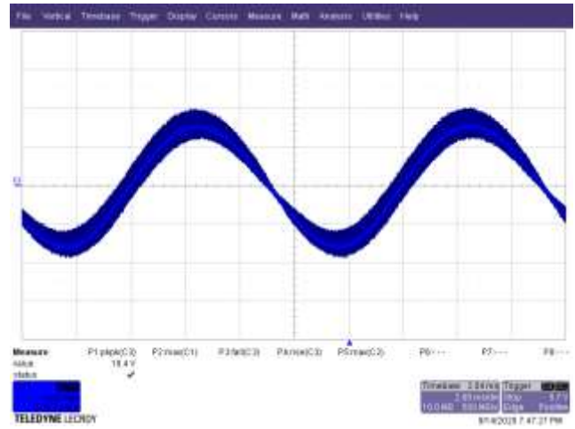
Figure 73 – Ripple, 230 VAC, 100% Load. 5 V / div., 2 ms / div.
