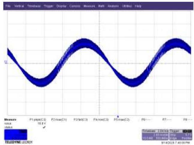
Figure 75 – Ripple, 264 VAC, 100% Load. 5 V / div., 2 ms / div.
