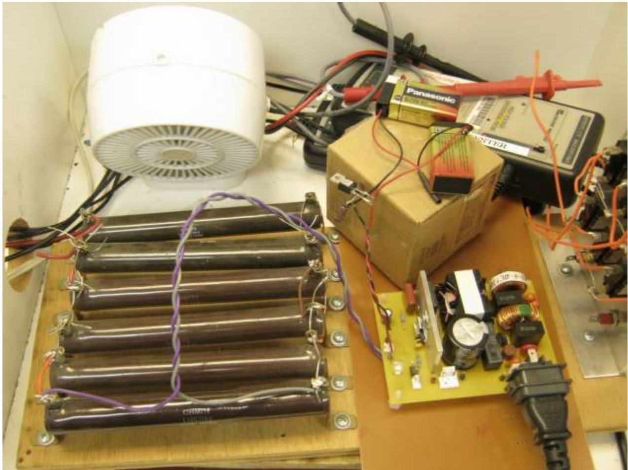
Figure 79 – Line Surge UUT Set-up.
