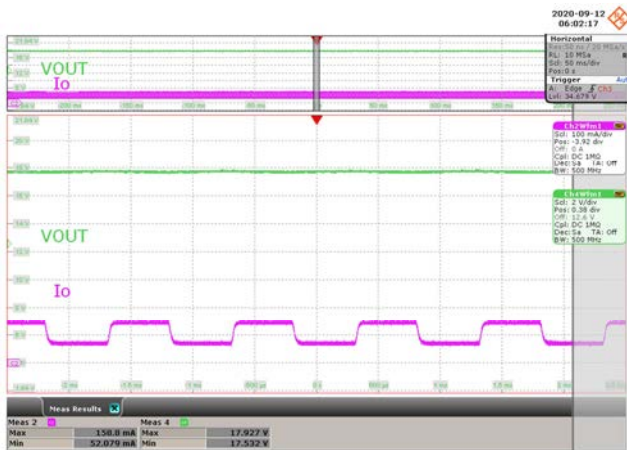
Figure 20 – 60 VDC Input. CH2: I_{OUT} , 100 mA / div., 50 ms / div. CH4: V_{OUT} , 2 V / div., 50 ms / div. Zoom: 500 \mu s / div. V_{OUT(MAX)} = 18.006 V, V_{OUT(MIN)} = 17.611 V.
