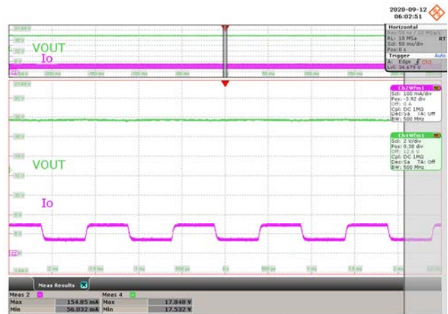
Figure 21 – 360 VDC Input. CH2: I_{OUT} , 100 mA / div., 50 ms / div. CH4: V_{OUT} , 2 V / div., 50 ms / div. Zoom: 500 \mu s / div. V_{OUT(MAX)} = 17.927 V, V_{OUT(MIN)} = 17.532 V.
