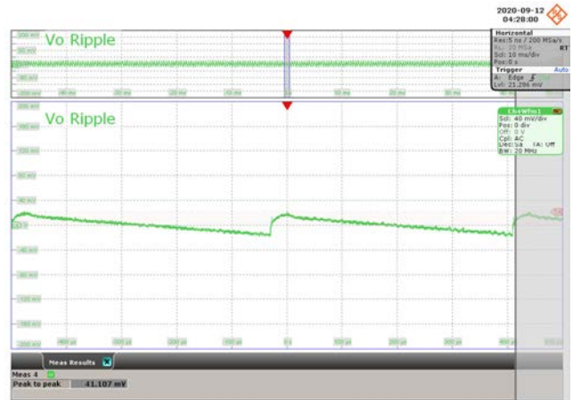
Figure 93 – 360 VDC Input. CH4: V_{OUT} , 40 mV / div., 10 ms / div. Zoom: 100 \mu s / div. 18 V Output Ripple = 41.10 mV.
