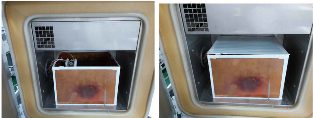
Figure 104 – Thermal Performance Set-up Using Thermal Chamber.
