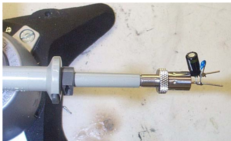
Figure 71 – Oscilloscope Probe with Probe Master ( www.probemaster.com ) 4987A BNC Adapter. (Modified with wires for ripple measurement, and two parallel decoupling capacitors added.)
