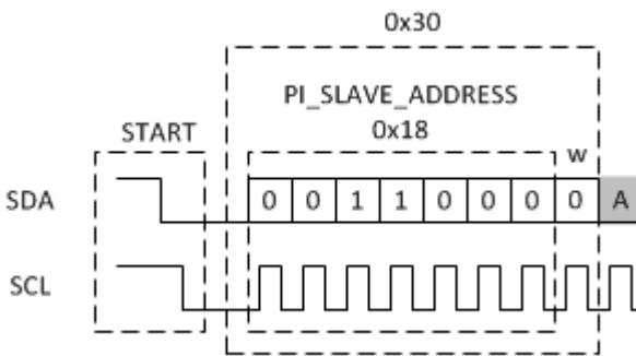
Then in the next I<sup>2</sup>C operation, a read request is sent to the slave and as a response to this request, the slave sends the Low Byte followed by the High Byte stored at the respective Telemetry register whose address was written to the Read Register. The first byte during this read operation of the I<sup>2</sup>C transaction is as follows
