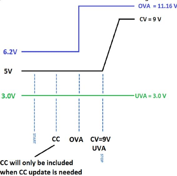
In the figure above, the command sequence is CC, OVA, CV, and UVA. The CC set-point will only be updated when requested. The example above shows that the OVA tracks the CV value. The OVA set-point is always 24% higher than the CV value.
