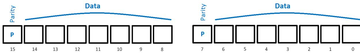
When converting the data into binary, the binary data starting from the 7<sup>th</sup> bit of the low byte must be shifted to the left by one place to reserve the position of the parity bit.
