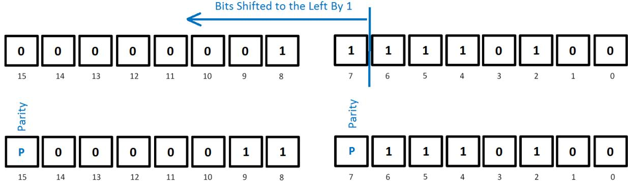
If the data has odd number of 1s, the parity bit is **0**, otherwise it is set to **1**.
