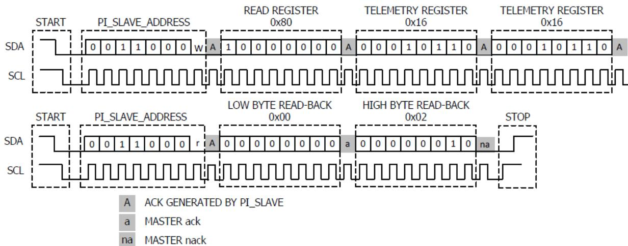
The address of the telemetry register from which data needs to be read, is first written to the Read Register which acts like a pointer to this telemetry register. The address of the Read Register is 0x80. Since the first operation while reading is a write operation, the first byte of the I<sup>2</sup>C transaction is as follows
