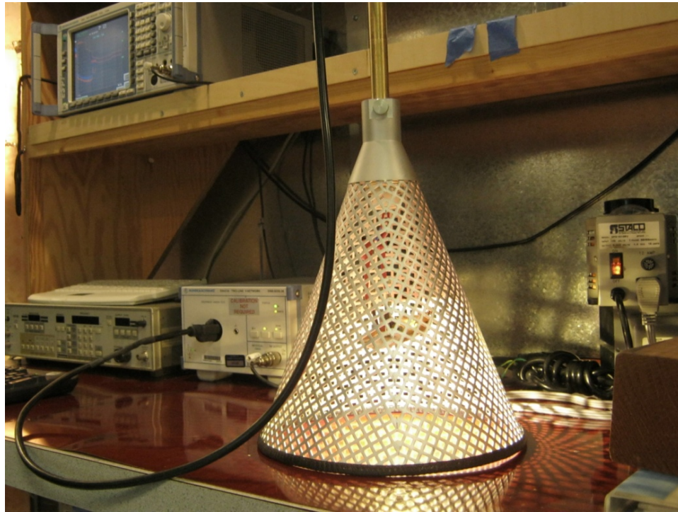
Figure 82 – EMI Test Set-up with the Unit and LED Load Placed Inside the Cone.
