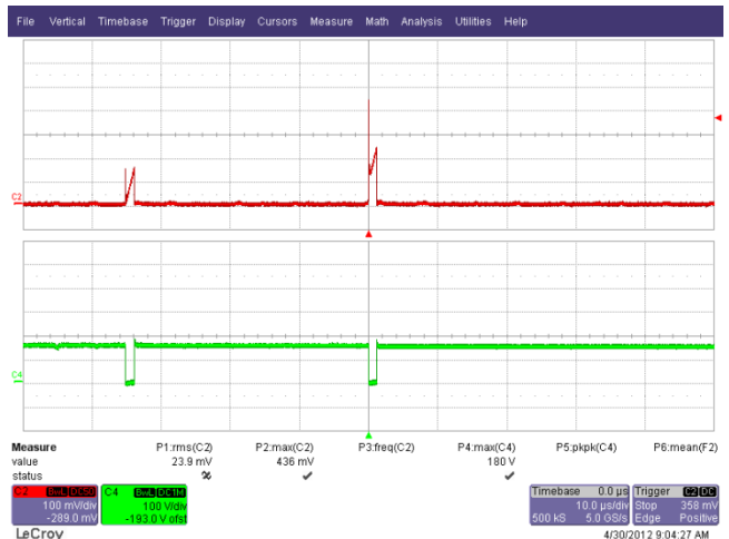
Figure 59 – 190 VAC, 50 Hz Output Short Condition. Upper: I_{DRAIN} , 100 mA / div. Lower: V_{DRAIN} , 100 V, 10 \mu s / div.
