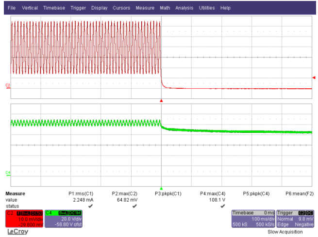
Figure 41 – 190 VAC Output Fall. Upper: I_{OUT} , 10 mA / div. Lower: V_{OUT} , 20 V, 100 ms / div.
