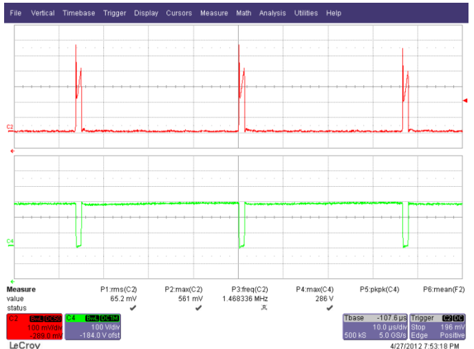
Figure 55 – 190 VAC, 50 Hz Start-up. Upper: I_{DRAIN} , 100 mA / div. Lower: V_{DRAIN} , 100 V, 10 \mu s / div.
