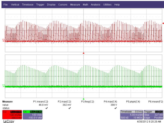
Figure 65 – 265 VAC, 50 Hz Output Short Characteristic. Upper: I_{OUT} , 100 mA / div. Lower: V_{PIV D2} , 100 V / div., 5 ms / div.
