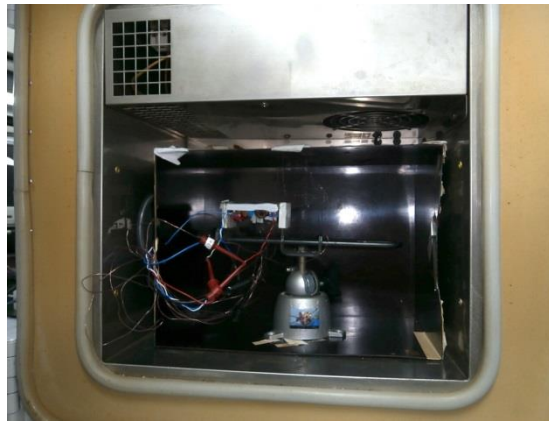
Figure 26 – Test Set-up Picture – Unit in Enclosure Placed Inside Thermal Chamber.
