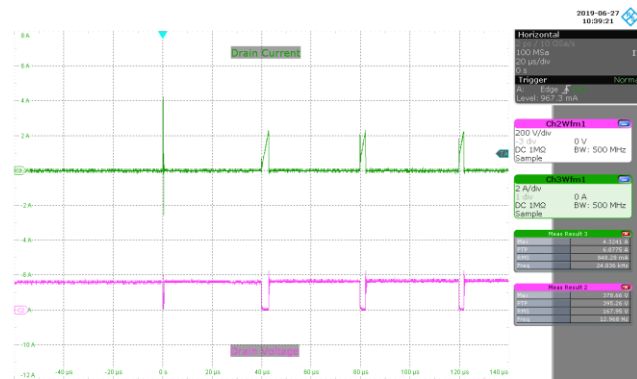
Figure 51 – 110 VAC 60 Hz, Full Load Start-up. Upper: I_{DRAIN} , 2 A / div. Lower: V_{DRAIN} , 200 V / div., 20 \mu s / div.
